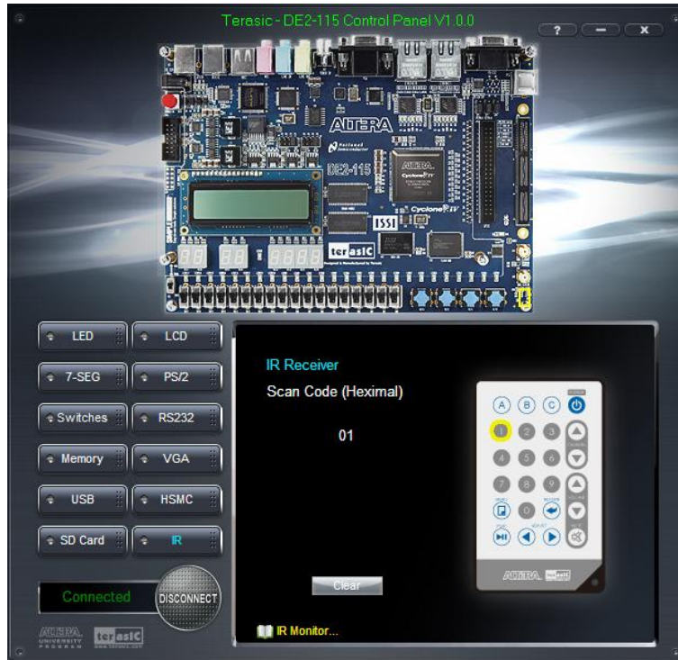
Figure 3-14 Testing the IR receiver using remote controller
