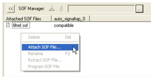
As you switch between configurations in the Data Log, you can extract the **SOF** that is compatible with that particular configuration. You can use the programmer in the SignalTap II Logic Analyzer to download the new **SOF** to the FPGA, ensuring that the configuration of your **.stp** always matches the design programmed into the target device.
