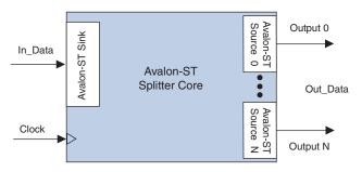
The Avalon-ST Splitter core copies all input signals from the input interface to the corresponding output signals of each output interface without altering the size or functionality. This include all signals except for the ready signal.
