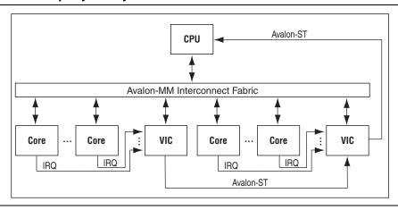
To use the VIC, the processor in your system needs to have a matching Avalon-ST interface to accept the interrupt information, such as the Nios® II processor's external interrupt controller interface.
