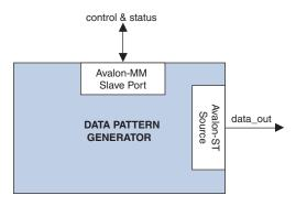
You can configure the width of the output data signal to either 32-bit or 40-bit when instantiating the core.
