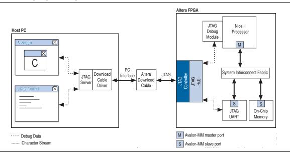
The JTAG controller on the FPGA and the download cable driver on the host PC implement a simple data-link layer between host and target. All JTAG nodes inside the FPGA are multiplexed through the single JTAG connection. JTAG server software on the host PC controls and decodes the JTAG data stream, and maintains distinct connections with nodes inside the FPGA.
