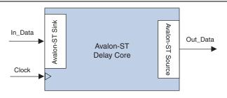
The Avalon-ST Delay core adds a delay between the input and output interfaces. The core accepts all transactions presented on the input interface and reproduces them on the output interface N cycles later without changing the transaction.
