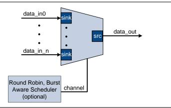
The internal scheduler considers one input interface at a time, selecting it for transfer. Once an input interface has been selected, data from that input interface is sent until one of the following scenarios occurs:
