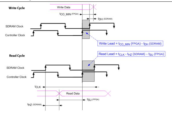
Figure 2–6. Calculating the Maximum SDRAM Clock Lead
