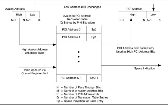
The address size selections in the translation table determine both the number of entries in the Avalon-to-PCI address translation table, and the number of bits that are passed through the transaction table unchanged.
