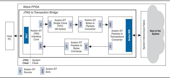
The SPI Slave to Avalon Master Bridge and the JTAG to Avalon Master Bridge cores accept encoded streams of bytes with transaction data on their respective physical interfaces and initiate Avalon-MM transactions on their Avalon-MM interfaces. Each bridge consists of the following cores, which are available as stand-alone components in SOPC Builder:
