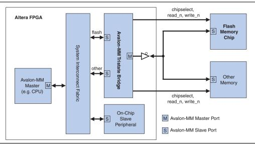
Avalon-MM master ports can perform read transfers directly from the CFI controller's Avalon-MM port. See "Software Programming Model" on page 4–4 for more detail on writing/erasing flash memory.
