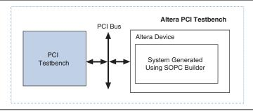
The simulation flow using Altera PCI testbench comprises the following steps.
