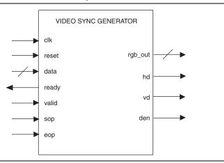
You can configure various aspects of the core and its Avalon-ST interface to suit your requirements. You can specify the data width, number of beats required to transfer each pixel and synchronization signals. See "Parameters" on page 27–2 for more information on the available options.
