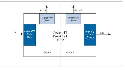
Figure 15-2. Avalon-ST Dual Clock FIFO Core
