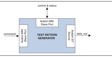
The data pattern is determined by the following equation: Symbol Value = Symbol Position in Packet XOR Data Error Mask. Non-packetized data is one long stream with no beginning or end.
