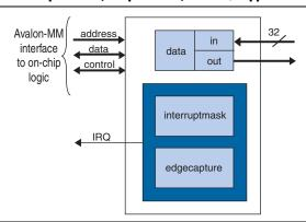
Figure 10–3 shows a block diagram of the PIO core configured in bidirectional mode, without support for IRQs.
