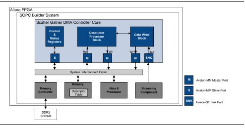
Figure 25–2 shows a different use of the SG-DMA controller core, where the core transfers data between an internal and external memory. The host processor and memory are connected to a system bus, typically either a PCI Express or Serial RapidIO $^{\text{TM}}$ .
