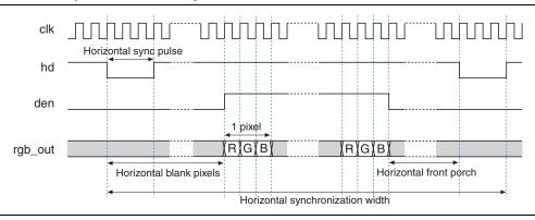
Figure 27–4 sho.ws the horizontal synchronization timing when the parameters **Data Stream Bit Width** and **Beats Per Pixel** are set to 24 and 1, respectively.
