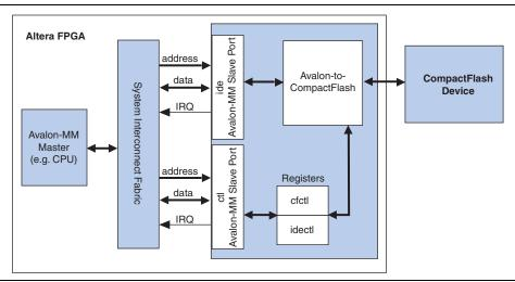
As shown in Figure 3–1, the CompactFlash core provides two Avalon-MM slave interfaces: the ide slave port for accessing the registers on the CompactFlash device and the ctl slave port for accessing the core's internal registers. These registers can be used by Avalon-MM master peripherals such as a Nios II processor to control the operations of the CompactFlash core and to transfer data to and from the CompactFlash device.
