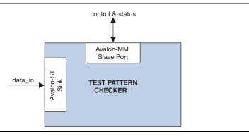
The test pattern checker core detects exceptions and reports them to the control interface via a 32-element deep internal FIFO. Possible exceptions are data error, missing start-of-packet (SOP), missing end-of-packet (EOP) and signalled error.
