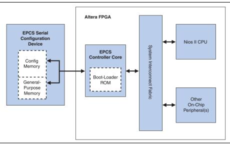
By virtue of the HAL generic device model for flash devices, accessing the EPCS device using the HAL API is the same as accessing any flash memory. The EPCS device has a special-purpose hardware interface, so Nios II programs must read and write the EPCS memory using the provided HAL flash drivers.
